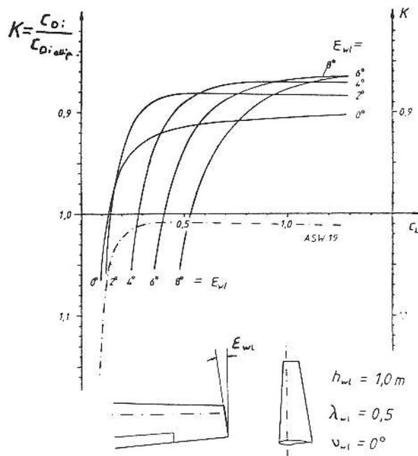
Fig. 4 Flight performances of the ASW-19 with winglets of different heights.
