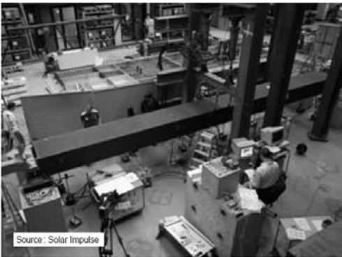
Figure 39 Wing box structure test.
