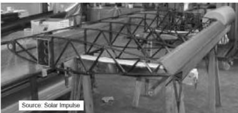
Figure 40 Horizontal tail, rib spar arrangement.
