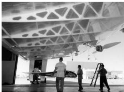
Figure 23 Wing structure of the Pathfinder (source AeroVironment)
