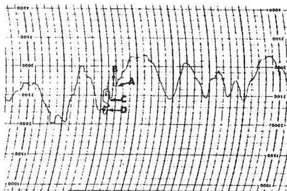
Figure 2—Microbarograph trace of part of the 21 August 1976 flight. Small time divisions are at 2 min intervals, and small height divisions are at 30 m intervals. The letters denote the following: A, first penetration through vertical portion of funnel; B, beginning of descent to lose height prior to second penetration through quasi-horizontal portion; C, beginning of second penetration; and D, end of second penetration.
