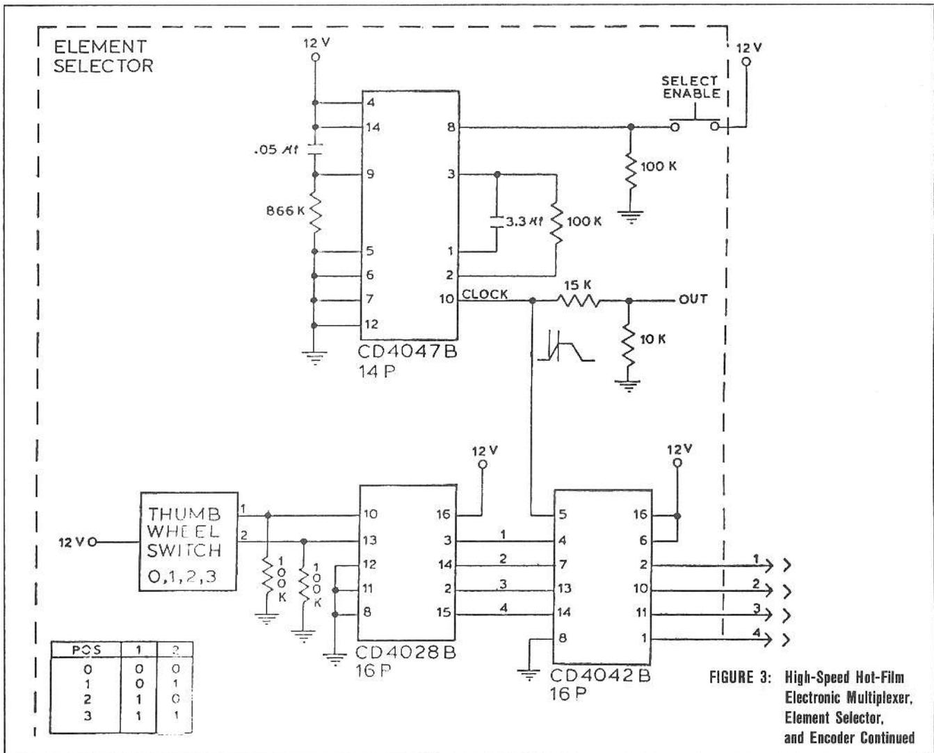
FIGURE 3: High-Speed Hot-Film Electronic Multiplexer, Element Selector, and Encoder Continued
