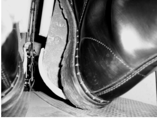
Figure 13 Foot reach to pedal impeded by panel.
