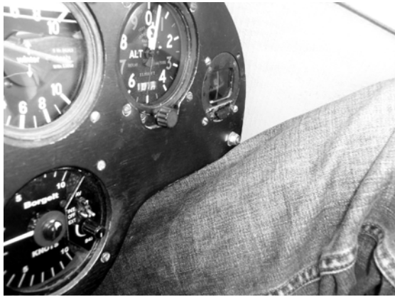
Figure 15 Instrument panel edge in leg contact.
