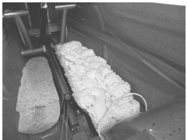
Figure 12 Cockpit floor raised for leg and heel support. .
