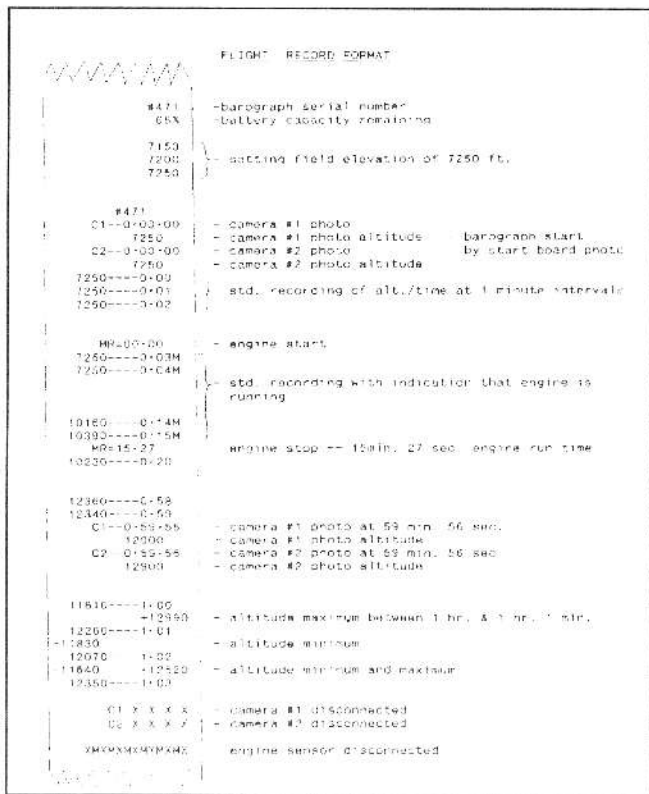
FIGURE 2. Annotated flight record tape showing the recording format for the various events.
