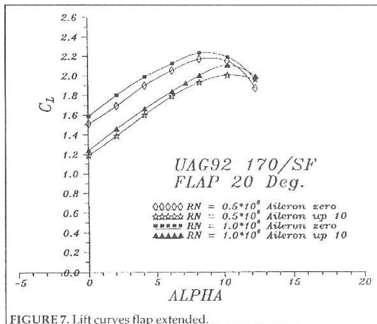
FIGURE 7. Lift curves flap extended.
