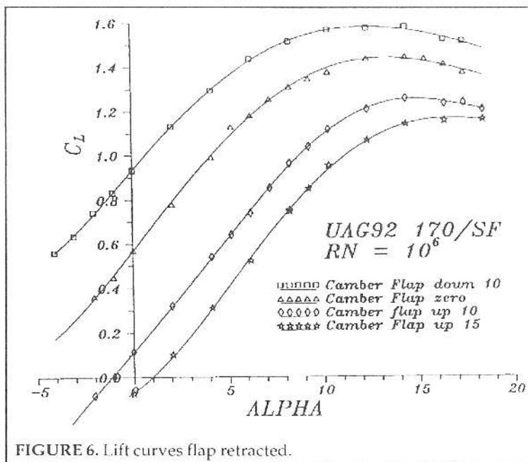
FIGURE 6. Lift curves flap retracted.
