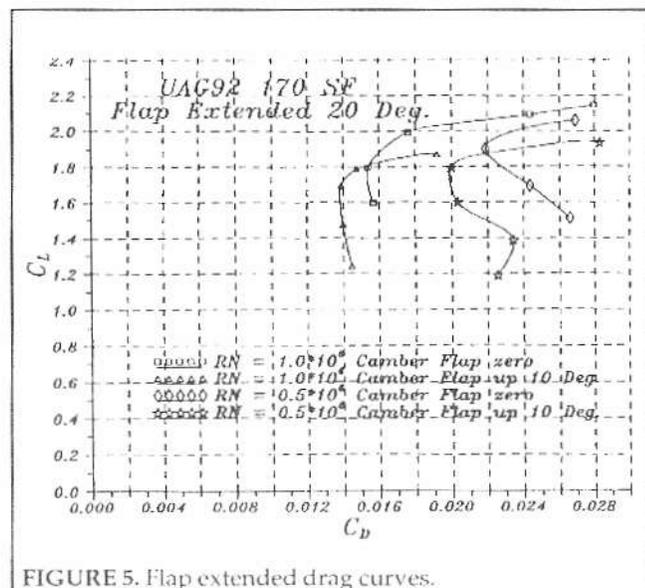
FIGURE 5. Flap extended drag curves.
