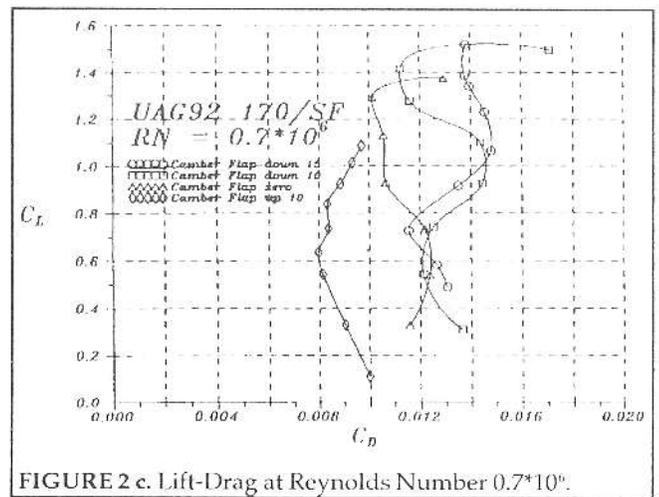
FIGURE 2 c. Lift-Drag at Reynolds Number 0.7\*10<sup>6</sup>.
