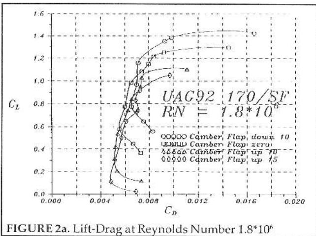
FIGURE 2a. Lift-Drag at Reynolds Number 1.8\*10<sup>6</sup>
