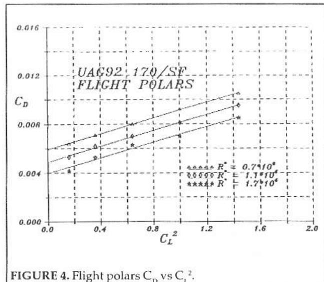
FIGURE 4. Flight polars  $C_D$  vs  $C_L^2$ .
