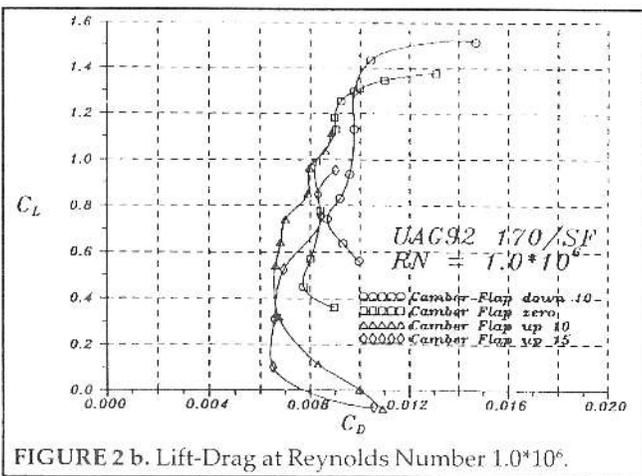
FIGURE 2 b. Lift-Drag at Reynolds Number 1.0\*10<sup>6</sup>.
