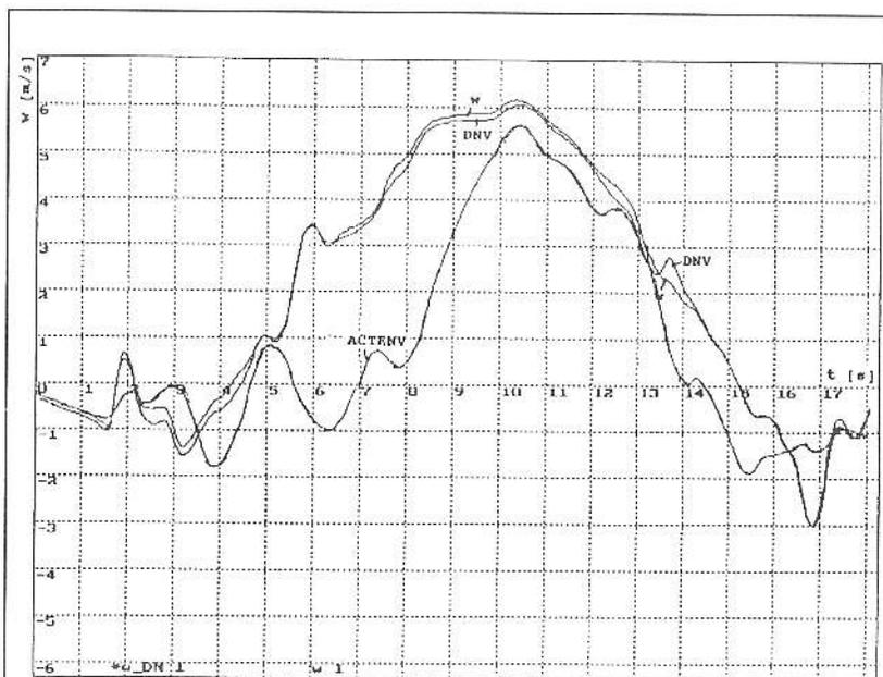
Figure 9. ACTENV readings; with turbulence; input  $T_c = 0$ ; tubing error correction; second order gust filter; output  $T_c = 0.75$  s; DNV readings; with turbulence; input  $T_c = 0$ ; tubing error correction
