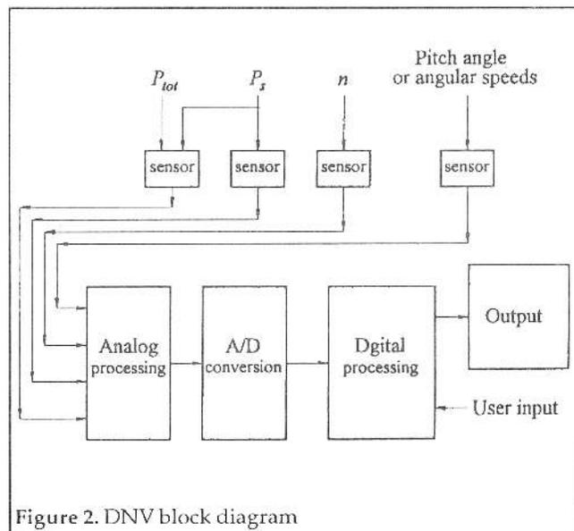
**Figure 2.** DNV block diagram
