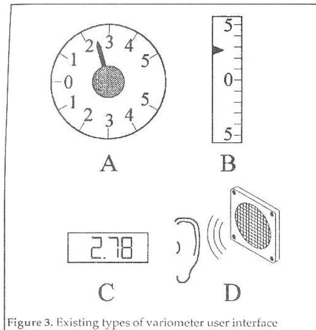
Figure 3. Existing types of variometer user interface
