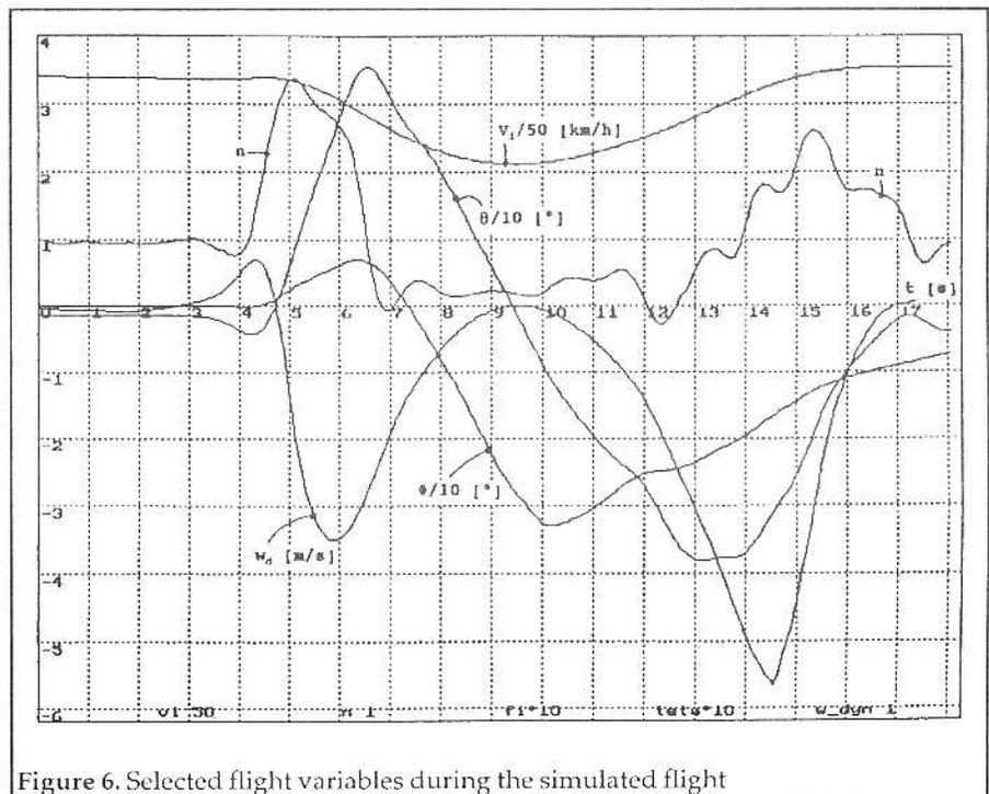
Figure 6. Selected flight variables during the simulated flight
