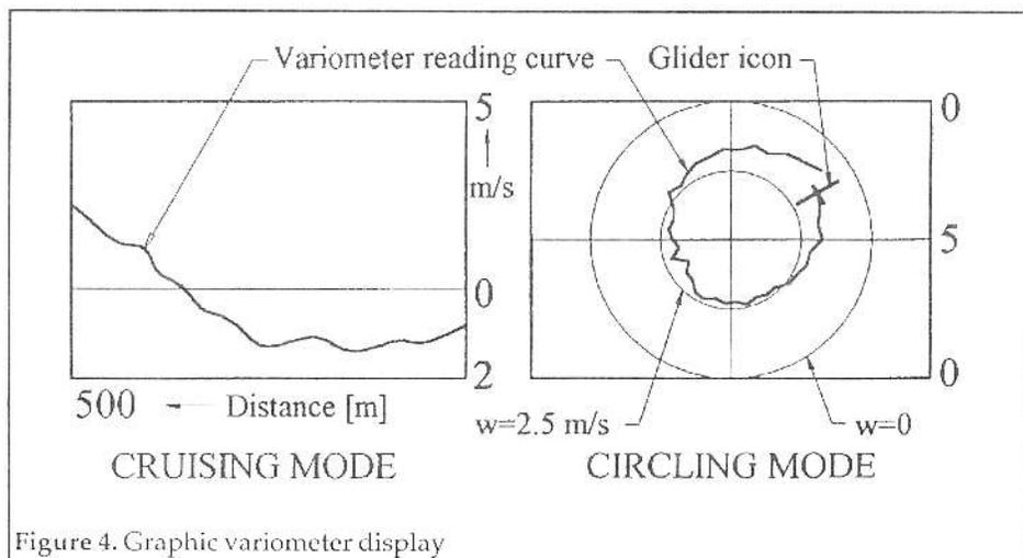
Figure 4. Graphic variometer display
