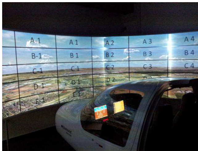
Fig. 3: Flight simulator cockpit with gridded projection screen.
