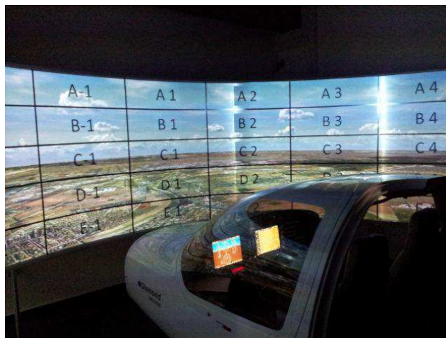
Fig. 3: Flight simulator cockpit with gridded projection screen.
