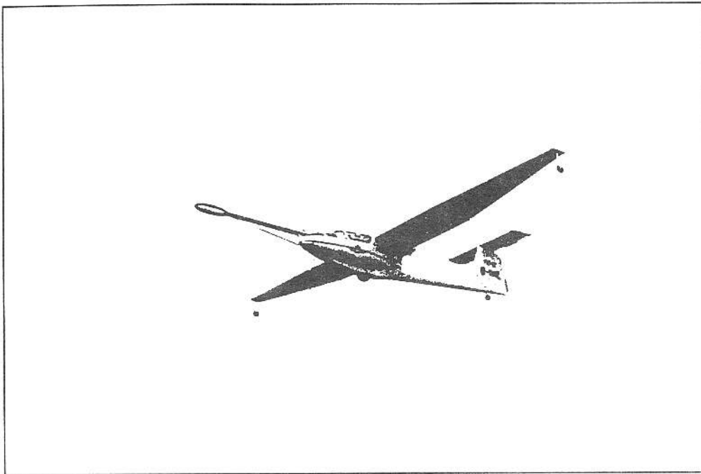
FIGURE 2. The SEAGULL SU-1, with the sensor mounted in front, far away from the metal construction.
