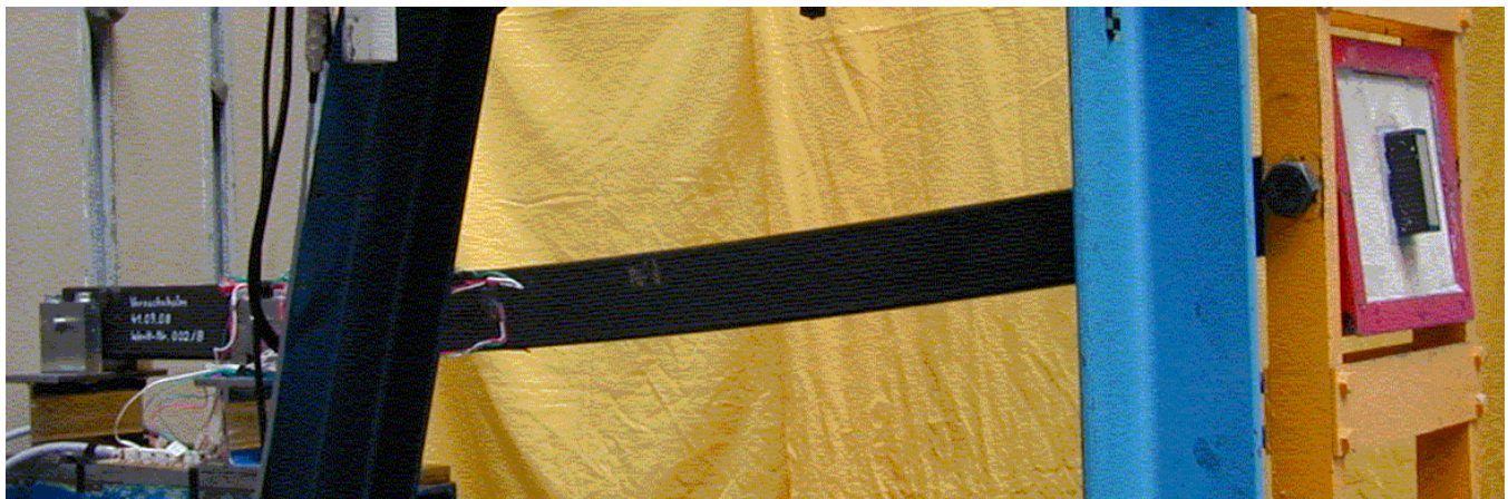
Figure 7 CFRP-spar in test bench at maximum load.
