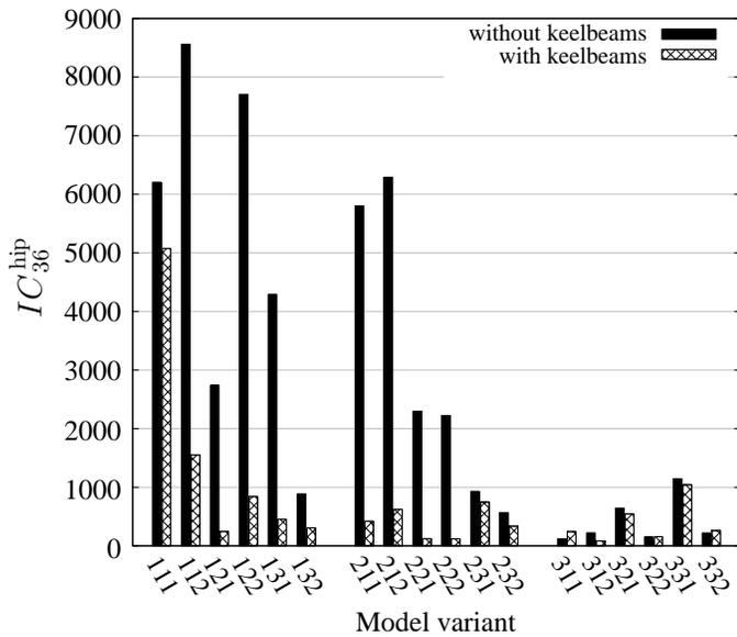
Fig. 8: Comparison of the rear occupant's  $IC_{36}^{\text{hip}}$
