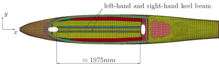
**Fig. 6: Integration of two keel beams (seat shells are not shown)**
