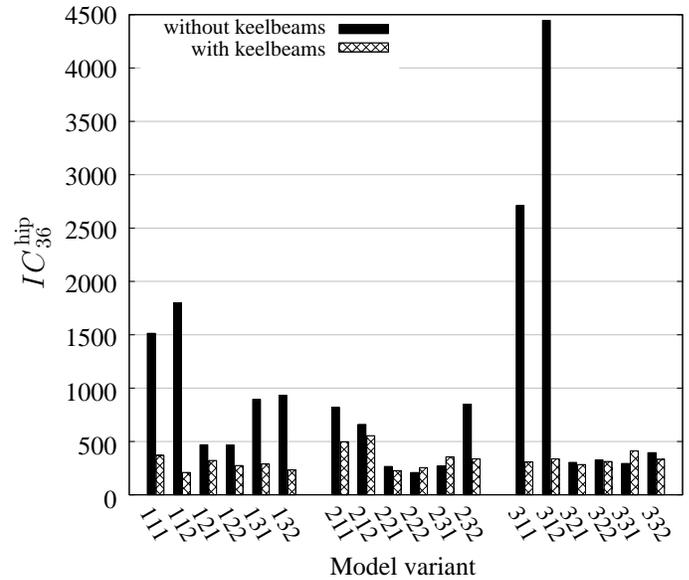
Fig. 9: Comparison of the forward occupant's  $IC_{36}^{\text{hip}}$
