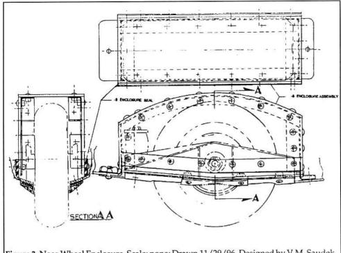
Figure 3. Nose Wheel Enclosure, Scale: none; Drawn 11/29/96, Designed by V.M. Saudek.
