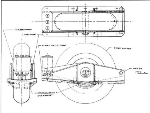
**Figure 1.** Three view Glider Nose Wheel with Brake, Scale: none; Drawn 11/29/96, Designed by V.M. Saudek.
