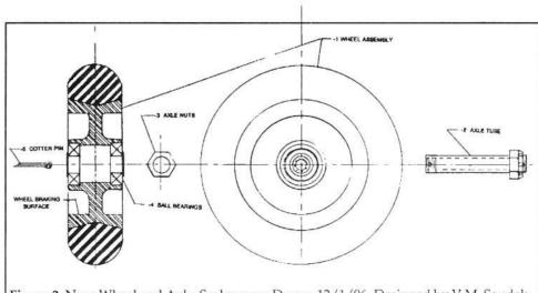
Figure 2. Nose Wheel and Axle, Scale: none, Drawn 12/1/96, Designed by V.M. Saudek.
