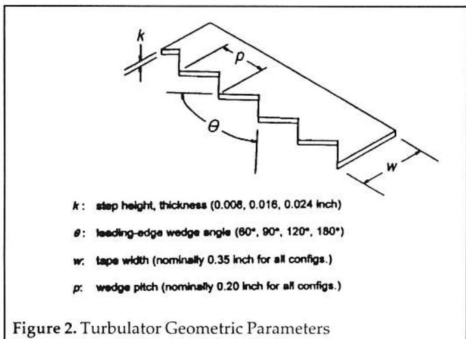
Figure 2. Turbulator Geometric Parameters
