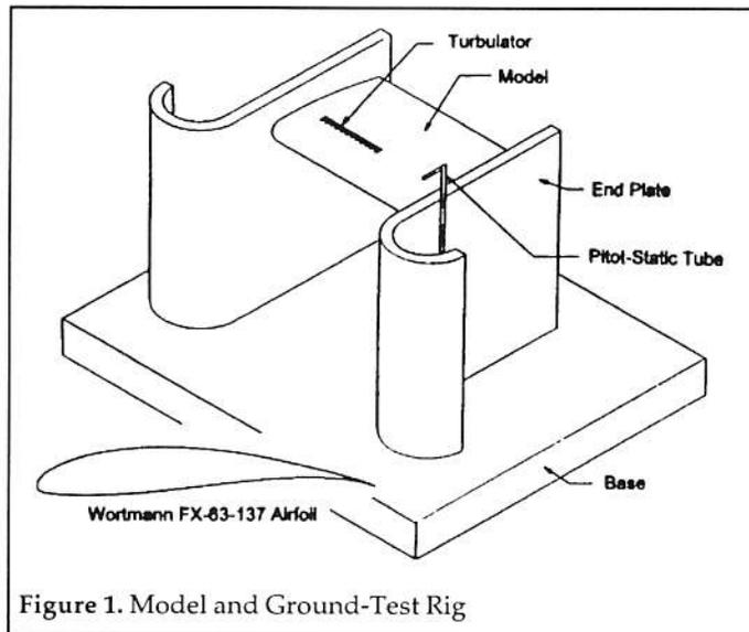
Figure 1. Model and Ground-Test Rig
