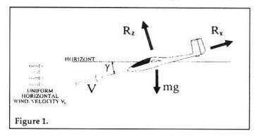
Using inertial Cartesian coordinates the equations of motion for a sailplane (Figure 1) becomes:
