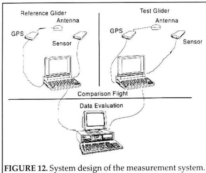
FIGURE 12. System design of the measurement system.
