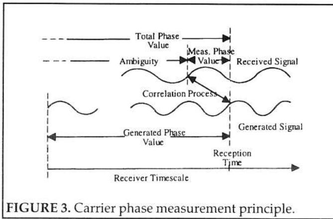
FIGURE 3. Carrier phase measurement principle.
