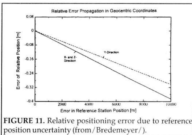
FIGURE 11. Relative positioning error due to reference position uncertainty (from /Bredemeyer/).
