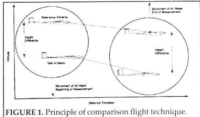
FIGURE 1. Principle of comparison flight technique.
