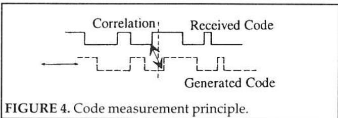
FIGURE 4. Code measurement principle.
