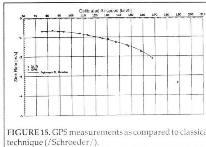
FIGURE 15. GPS measurements as compared to classical technique (/Schroeder/).
