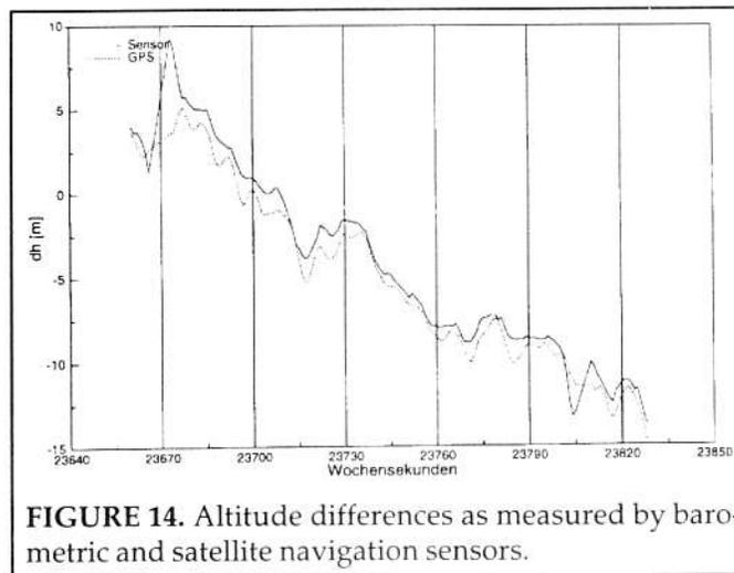
FIGURE 14. Altitude differences as measured by barometric and satellite navigation sensors.
