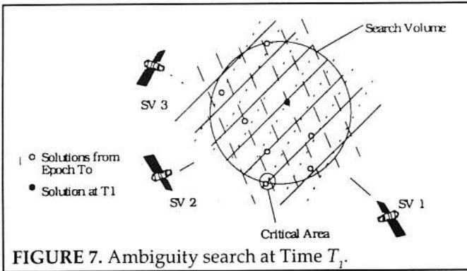
of the search volume. One can now use the change of geometry caused by the movement of the satellites with time to eliminate further possibilities, until only the correct solution remains (Figure 7).
