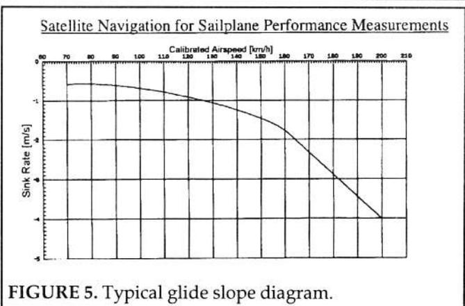
FIGURE 5. Typical glide slope diagram.
