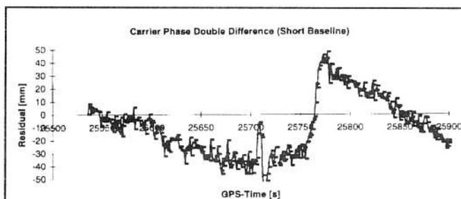
FIGURE 10. Low-cost receiver carrier noise.
