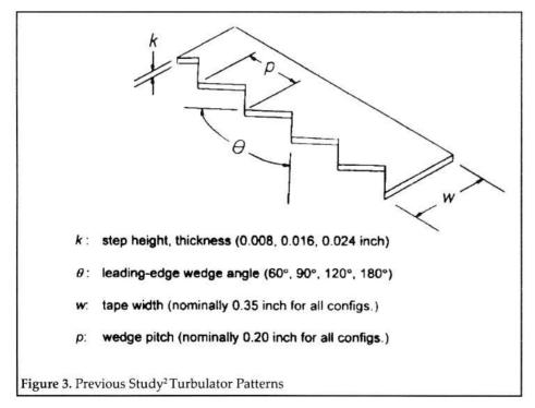
leading edge with either a straight trailing edge, or on both leading and trailing edges. While the previous study<sup>2</sup> examined 60°, 90°, 120°, and 180° (flat) leading-edge wedge angles (Figure 3), the current study incorporated the testing of six different patterns as shown in Figure 4 (the flow
