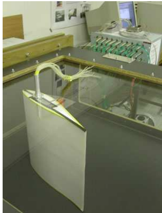
Figure 4 Model of airfoil FX66-17AII-182 in test section of open circuit wind tunnel with closed test section.
