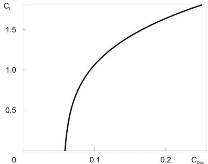
**Figure 3** Drag polar of motor glider with extended engine.
