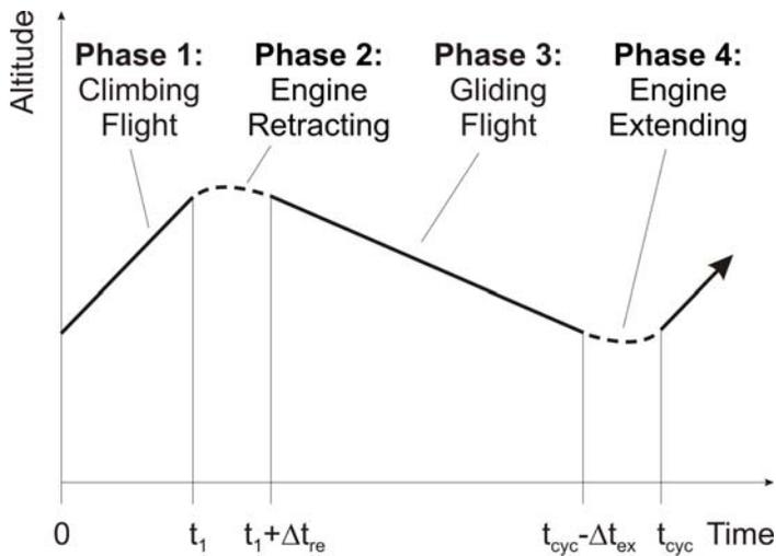
**Figure 4** Structure of optimal saw-tooth flight mode for range maximization.
