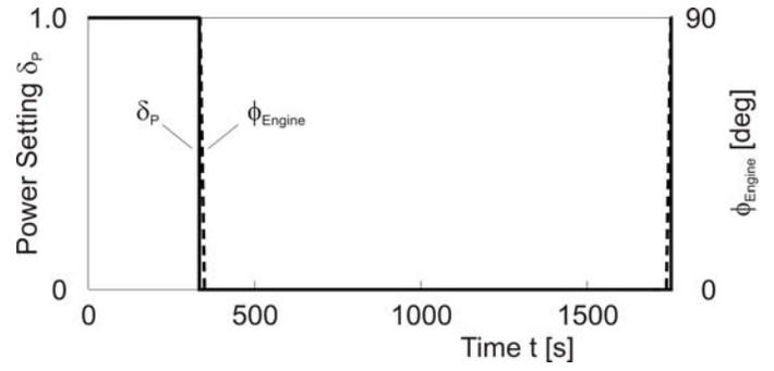
**Figure 11** Optimal time histories of power setting and engine inclination angle.
