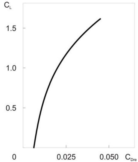
**Figure 2** Drag polar of motor glider with retracted engine.
