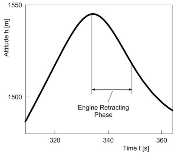
**Figure 7** Optimal transition flight maneuver from climb to glide.
