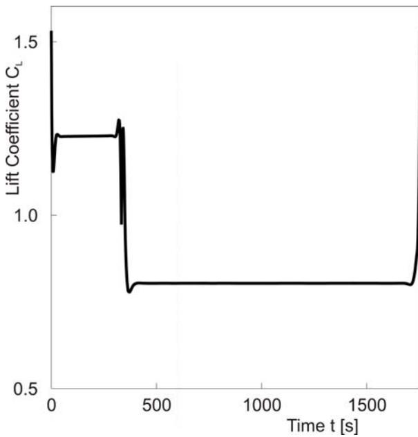
**Figure 10** Optimal lift-coefficient time history.
