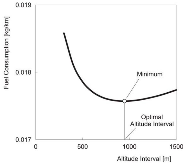
**Figure 12** Effect of altitude interval of saw-tooth cycle on fuel consumption.
