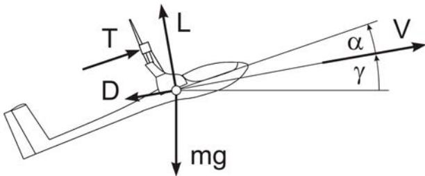
**Figure 1** Forces acting on motor glider with extended engine.
