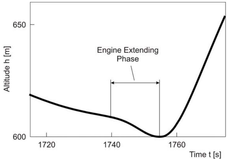
**Figure 8** Optimal transition flight maneuver from glide to climb.
