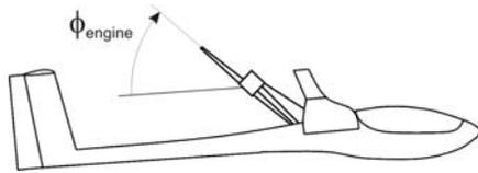
**Figure 5** Inclination angle of engine.
