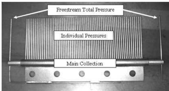
Figure 7 Integrating wake rake built at Saint Louis University.
