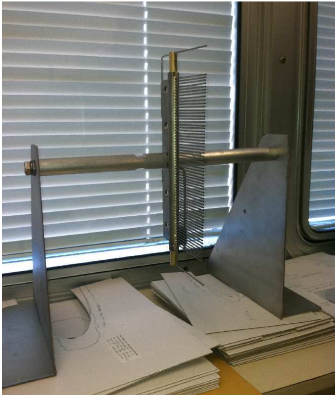
Figure 9 Integrating wake rake and its mounting behind wing.
