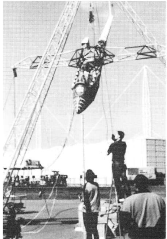
Fig. 19: Crash test at FH Aachen on a sailplane dummy with hybrid nose of the cockpit (photo by courtesy of W. Röger)
