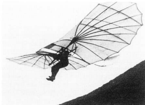
Fig. 1: Lilienthal with his "Normal Sailing Apparatus" from 1894 achieving distances of 80 m from a height of about 15 m
