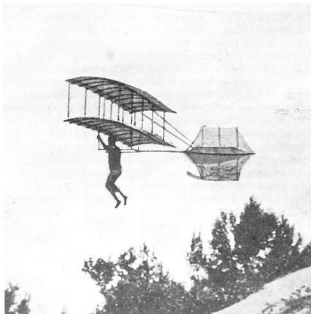
Fig. 11 The Chanute-type biplane in flight. Photo probably taken on 11 September 1896. From National Air and Space Museum (NASM negative no. 1A-20359).
