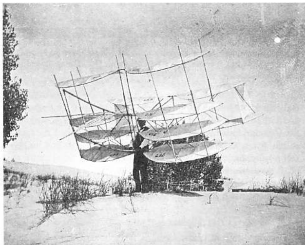
Fig. 10 Octave Chanute, "getting the feel for it!" Note numbering of each wing of "Katydid" multiple wing glider. From Octave Chanute Papers , Library of Congress, Washington, DC.
