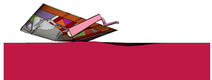
Fig. 24: Desired behavior of the nose cone of the fuselage at deformable barrier impact.
