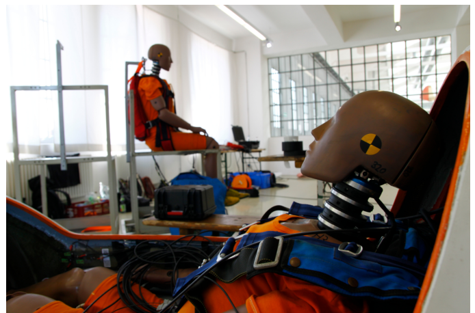
Fig. 6: 50th percentile male dummies prior to the crash test.
