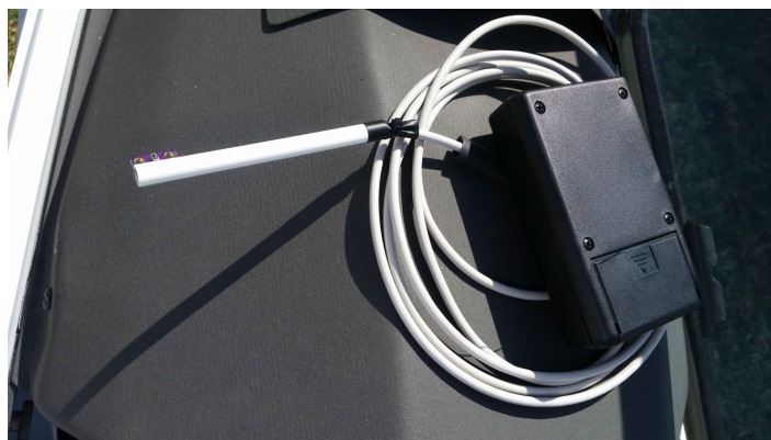
Fig. 2: Measurement hardware installed on the Ventus-2 glider.
