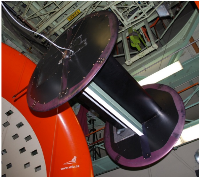
Fig. 2: Model equipped with the extended airbrake in the test section.
