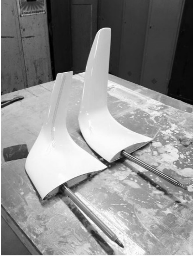
Fig. 11: Baseline SB 14 winglet (left), the reference for the performance flight tests conducted, and the optimized SB 15 winglet (right).
