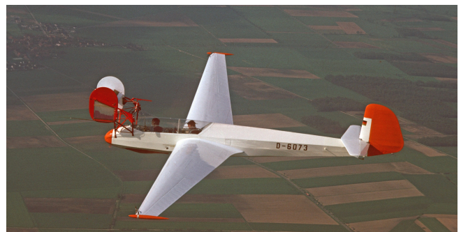
Fig. 27: Free-flight airfoil testing.
