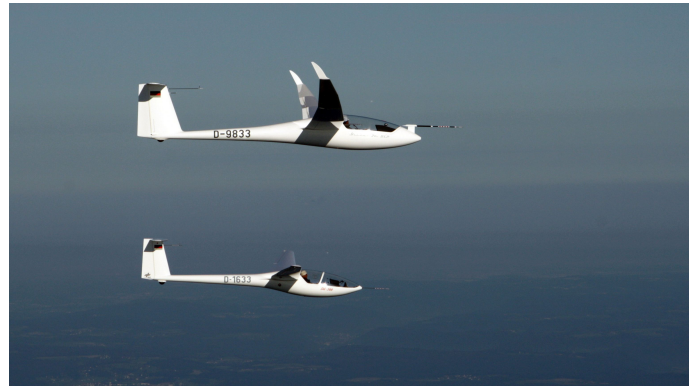
Fig. 47: The “holy” reference glider Discus 2c-DLR in formation with its predecessor, the DG 300/17, during a test run.
