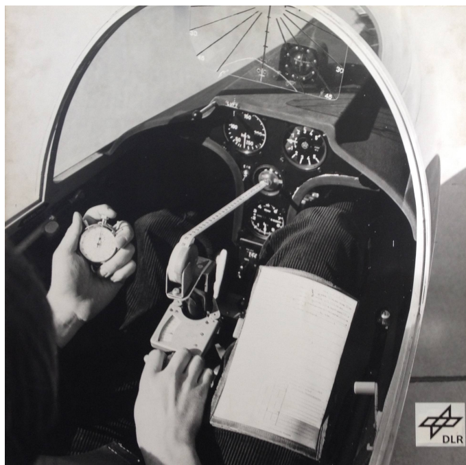
Fig. 42: Cockpit with very simple test tools used for “Zachern”.
