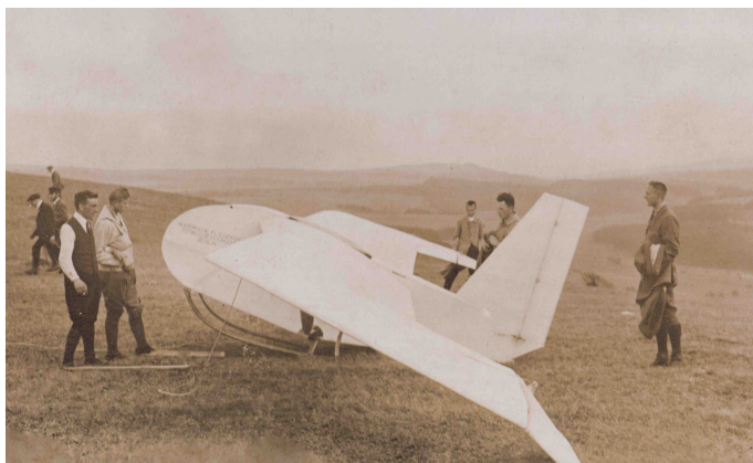
Fig. 36: B 1, one of the early tailless glider designs.
