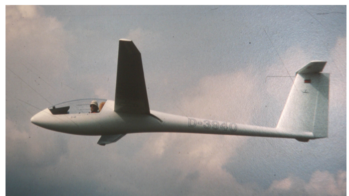
Fig. 31: D 40 "pocket-knife-wing-flaps" retracted.
