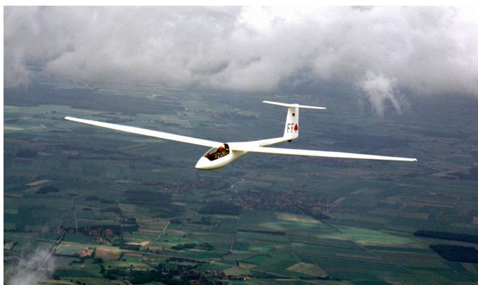
Fig. 29: SB 11, the first glider with an all carbon-fibre structure, in flight.
