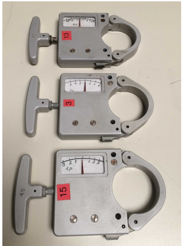
Fig. 45: Hand forces for pitch and roll control are measured using spring scales.
