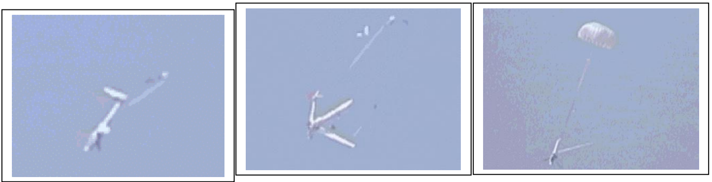
Figure 14 Separated wings due to the pitch rotation MISTRAL C, Vne
