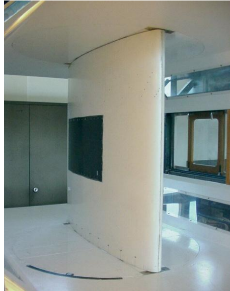
Figure 7 Wind tunnel model for boundary layer suction experiments.
