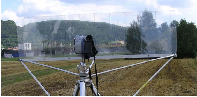
Figure 9 Example of a ground equipment for take-off and landing test. A camera is looking through a transparent grid. It requires a very precise setup.
