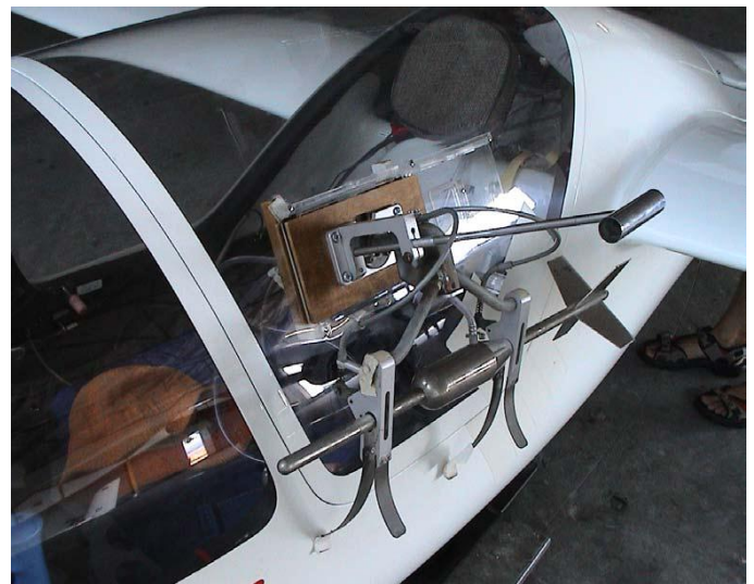
Figure 2 Deployable static probe used for calibration of the static system
