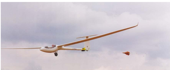
Figure 5 Drag chute for spin tests after use, partly released to reduce drag
