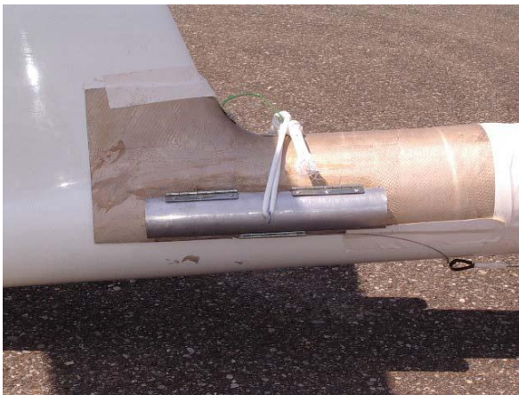
Figure 4 Jettisonable ballast for spin tests
