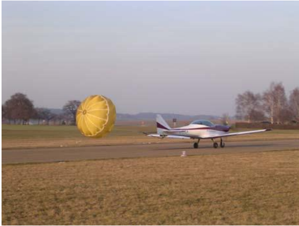
Figure 3 Drag chute for spin tests
