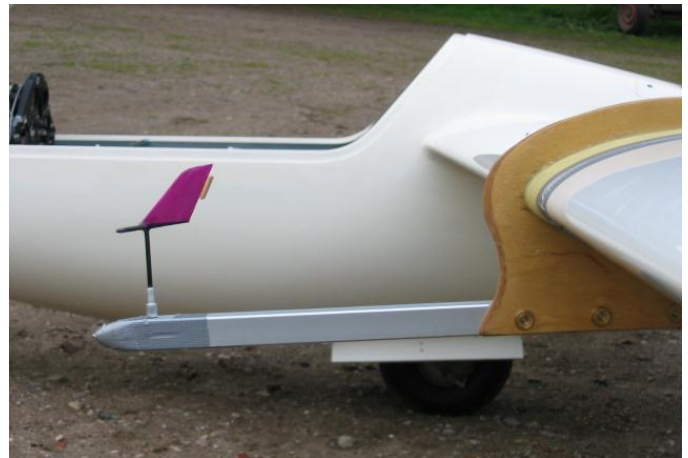
Figure 1 Wind vane installed in front of the ASW-19BX wing.
