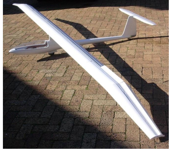
Figure 6 Anhedral of the outer wing panels and the upper-surface-only aileron-spoilers extended on the port wing.
