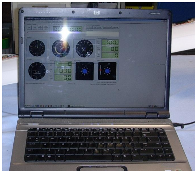
Figure 3 Personal computer displaying inflight data telemetered from the model.
