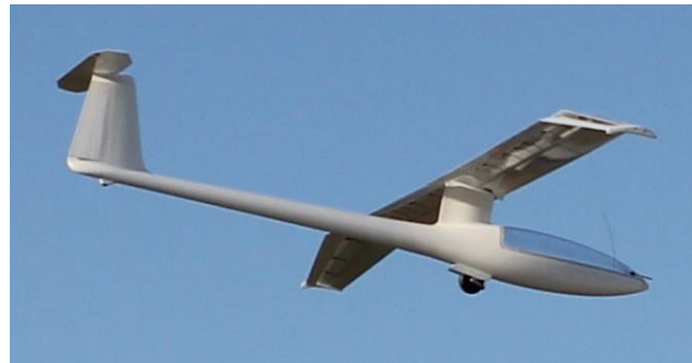
Figure 2 Quarter-scale model of the J-5 in flight.
