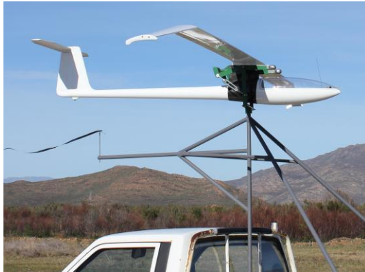
Figure 5 Rig for flight-performance analyses.
