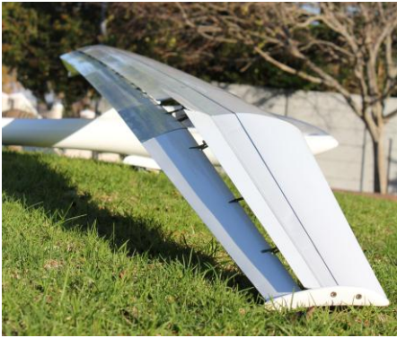
Figure 4 (Top) Fowler flap retracted, (Bottom) Fowler flap extended.
