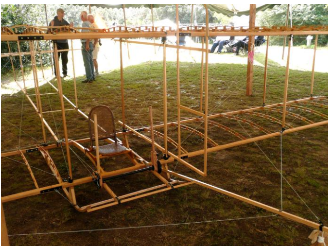
The replica 1911 Wright replica started by the late Jim Dayton and partially finished by friends and members of his family. Note upright pilot seating. Visitors to Jockey's Ridge enjoyed trying the wing warping and unique Wright controls. (Photo credit: Paul Rabourn).
