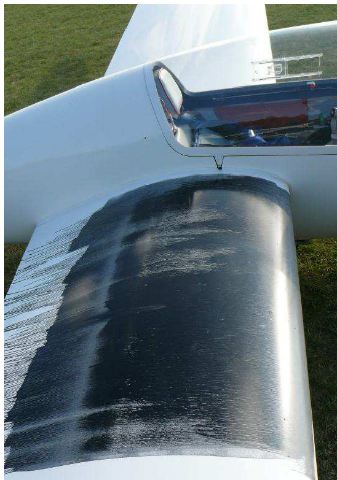
Fig. 6: Flow visualization in free flight, Twin-Astir with Eppler 603 airfoil.
