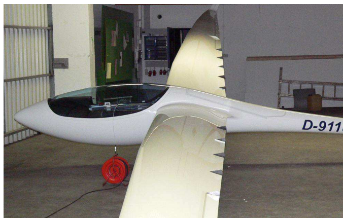
Fig. 1: ASW 28 carrying 5 pairs of fences
