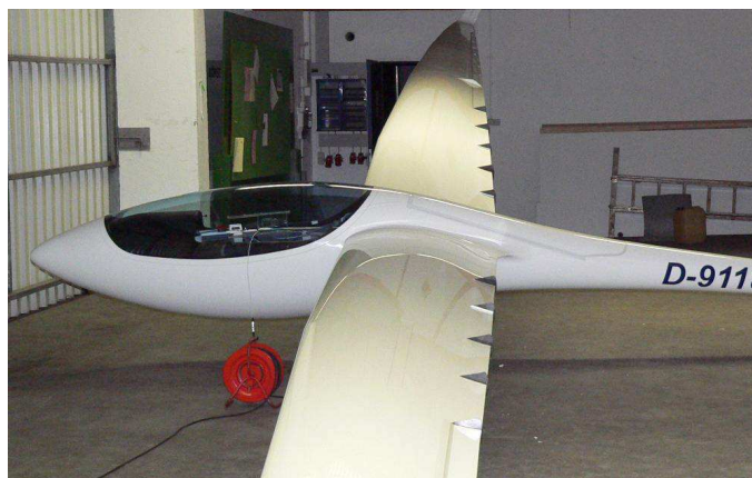
Fig. 1: ASW 28 carrying 5 pairs of fences
