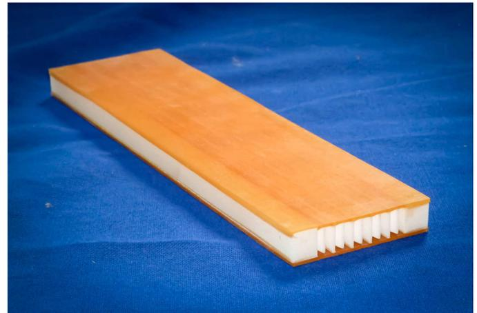
**Fig. 13: Sandwich with accordion honeycomb core and silicone top layers [21].**
