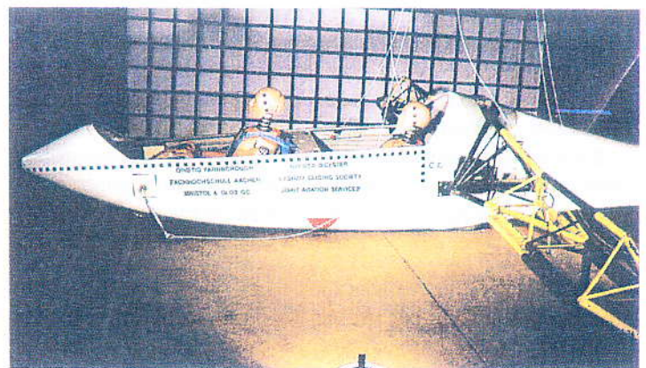
The glider after the final test, when the structure broke. The girders, borrowed from Germany and brought to the UK on a car roofrack, simulated the weight of wings.
