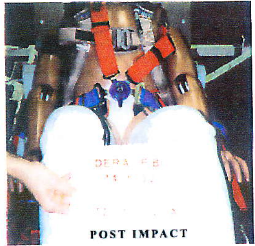
After impact, the shoulder and lap straps are out of position. There is potential for serious injury to be caused to the vulnerable abdomen by the movement of the lap strap.
