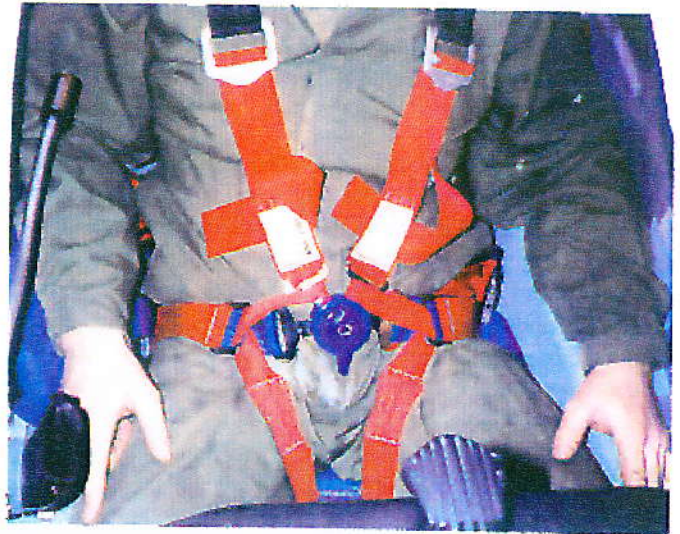
This six-point harness has two lap straps, two shoulder straps and two crotch straps. But how does it perform in simulated crashes and in flight?
