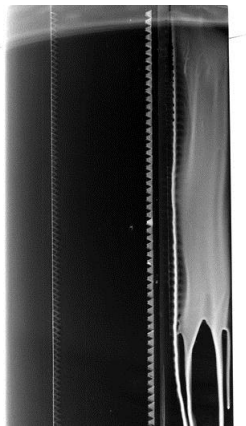
Figure 10 Oil visualization of the controlled case (low-profile rectangular VGs, x_2 , \Delta z_2 ), with zig-zag tape and with flap deflection (the free stream flow direction is from left to right).
