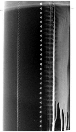
a) Figure 9 Oil visualization of the controlled case (low-profile rectangular VGs, x_1 , \Delta z_1 ), with zig-zag tape and with flap deflection (the free stream flow direction is from left to right).
