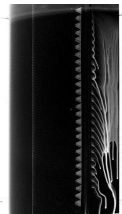
b) Oil visualization of the controlled case (conventional rectangular VGs, x_2 , \Delta z_2 ), with zig-zag tape and with flap deflection (the free stream flow direction is from left to right).
