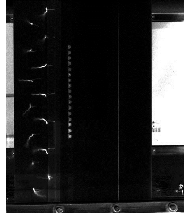
b) Controlled case (conventional triangular VGs, x_1, \Delta z_2 ) without flap deflection, \alpha = 15 deg. (the free stream flow direction is from right to left).
