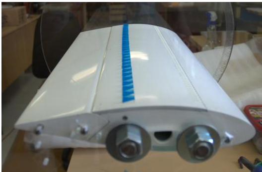
Figure 3 VGs location on upper surface of the model.
