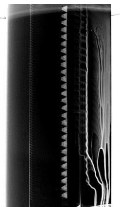
a) Figure 11 Oil visualization of the controlled case (conventional rectangular VGs, x_1 , \Delta z_2 ), with zig-zag tape and with flap deflection (the free stream flow direction is from left to right).
