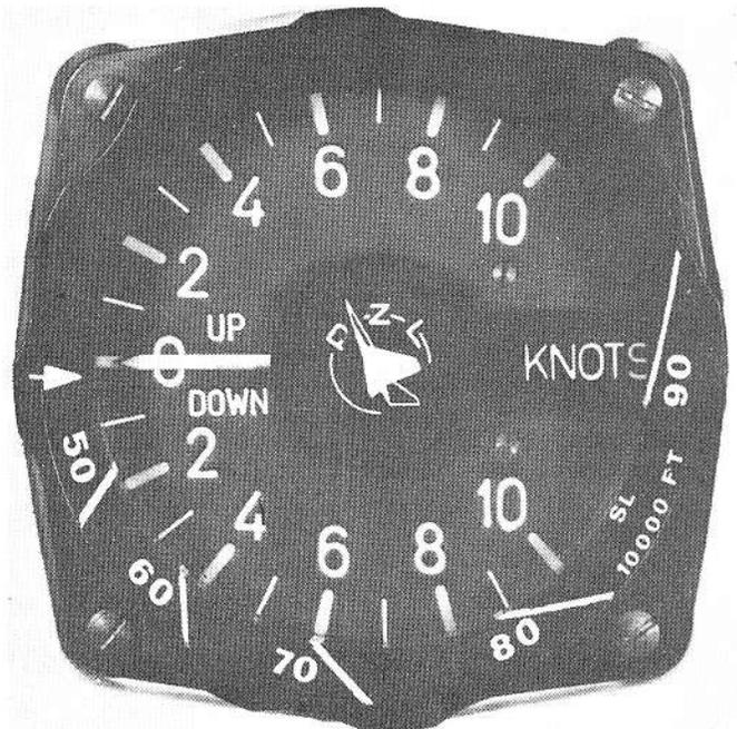
FIGURE 2. Perhaps a more practical arrangement. The inner edge of the verge ring is calibrated for sea-level, the outer edge for 10,000 ft. Approximate interpolation for other heights should be good enough. The calibration is for the "Standard Libelle."
