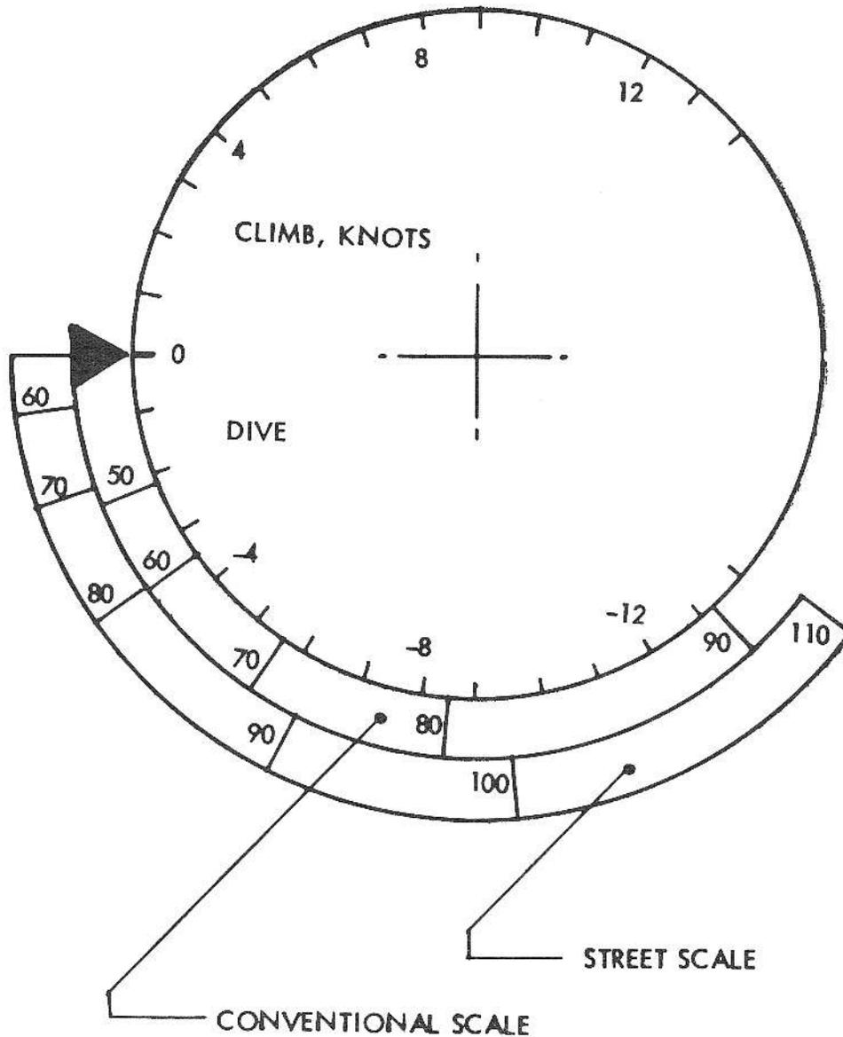
FIGURE 3. Two-Scale Speed Ring
