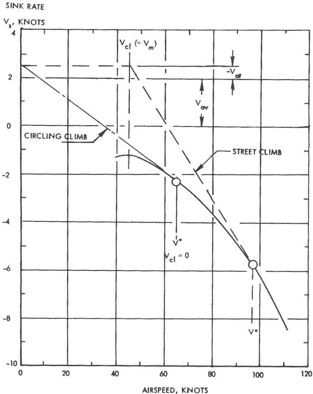
FIGURE 2. Graphical Solution for Optimum Cruise Speed  $V^*$  Standard Class Glider
