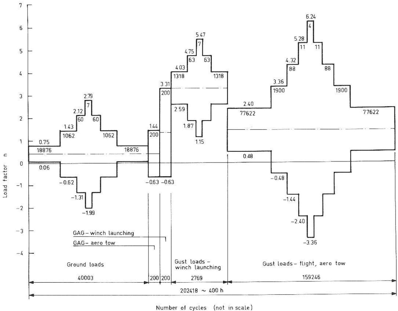
Figure 3. PIK-20D fatigue testing program (400 hours block)
